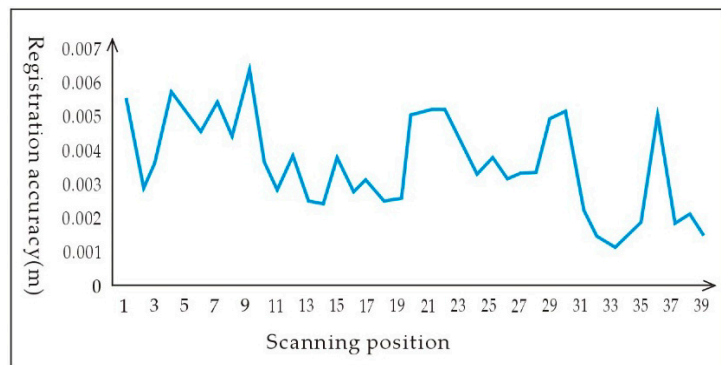
Figure 4. Registration accuracy map adjacent scanning positions.
