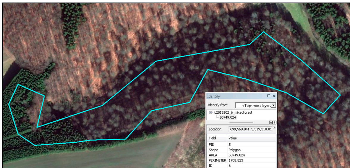
Figure 1. A 0.7 by 0.3 km area with a seemingly faulty reference polygon (center coordinates 49^{\circ}47'37''\text{N} , 5^{\circ}46'28''\text{E} ), which was labelled as mixed forest but that appears to be mostly covered by deciduous trees in the backdrop, which is a leaf-off image from Google Earth.
