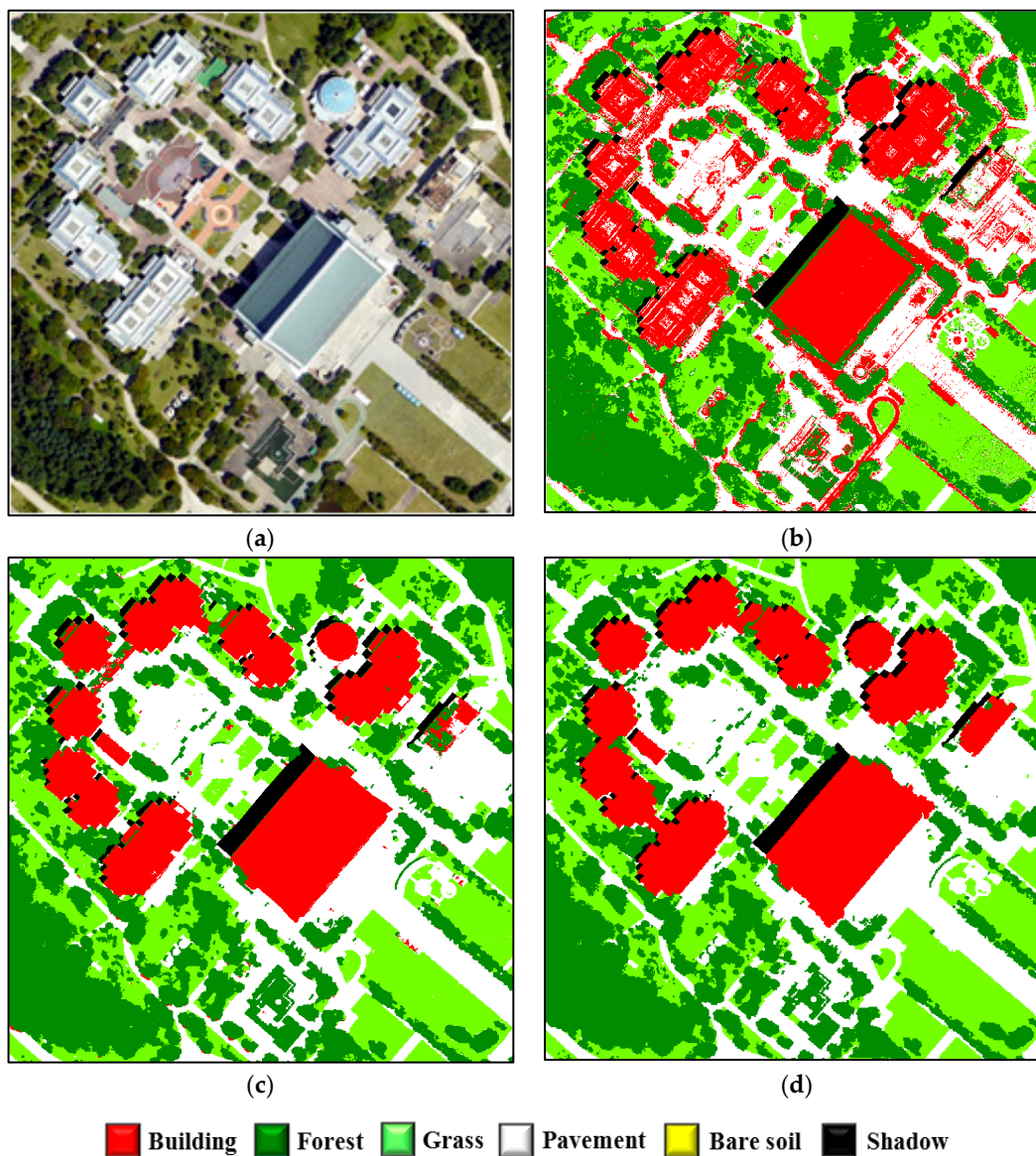
Figure 6. Final results for site 1: (a) aerial image; (b) Max-Min method; (c) SSI, nDSM method; and (d) the new method.
