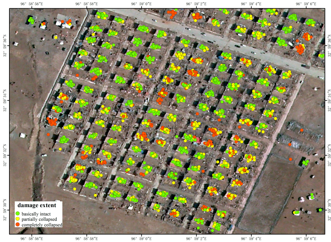
Figure 4. The experiment area and the location of the 3456 data points, which were contributed by 27 participants online. In the map, the green, yellow and red points indicate the damage type of “basically intact”, “partially collapsed” and “completely collapsed”, respectively.
