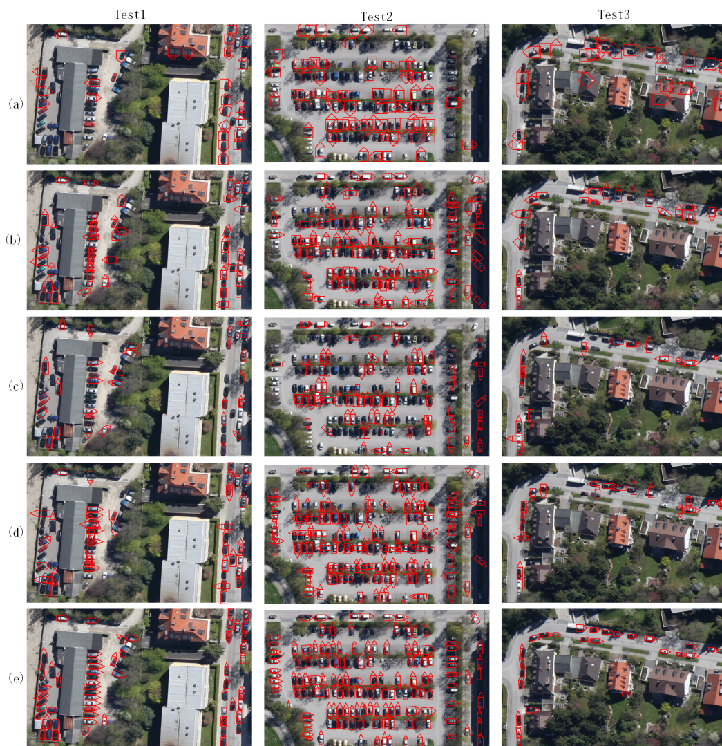
Figure 4. Detection results of different methods for three image blocks on DLR Vehicle Aerial dataset. The red box denotes correct localization, and the triangle represents the direction of the vehicle. (a) The results on the first row are detected by the aggregated channel feature (ACF) detector. (b) The second row is FRCN_VGG (VGG-16 based Faster R-CNN, FRCN_VGG). (c) The third row is YOLO2 (You Only Look Once, YOLO). (d) The fourth row is SSD512 (Single Shot MultiBox Detector, SSD). (e) The bottom row is Oriented_SSD512.
