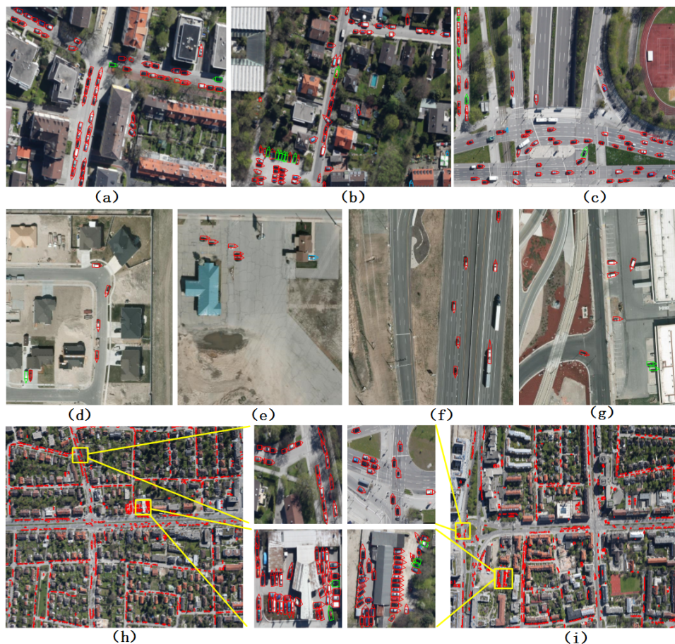
Figure 8. Detection results of our method Oriented_SSD512. A red box denotes correct localization; a blue box denotes false alarm; and a green box denotes missing detection. (a–c) are image blocks of DLR Vehicle Aerial test aerial images; (d–g) are VEDAI512 images; (h,i) are the original large aerial images of the DLR Vehicle Aerial dataset.
