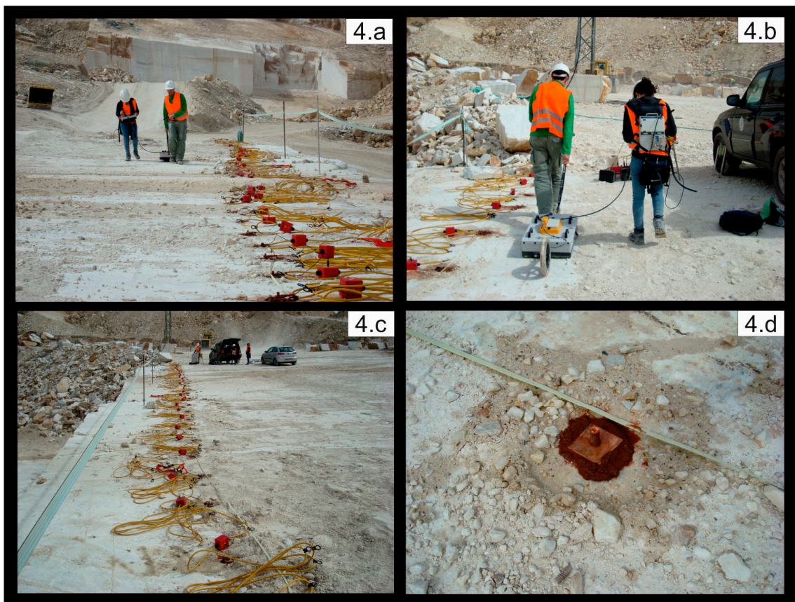
Figure 4. (a) GPR profile performed on the marble bench; (b) Detail from the 250 MHz antenna on the bank; (c) Position of the ERI profile on the primary bank; (d) Detail of a copper electrode and clay.
