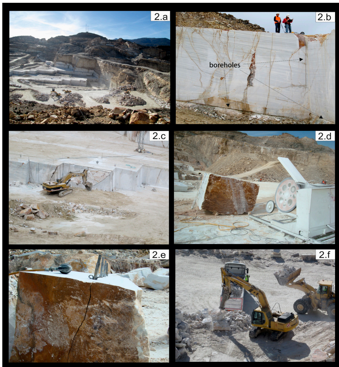
Figure 2. (a) Overview of the quarry; (b) Details of the three perpendicular holes that delineate the secondary bank; (c) Cutting of tertiary blocks with a diamond wire (detail of the block is outlined). Excavator extracting blocks over the sand bed. Note the breakage along a fracture plane; (d) Squaring a block with a diamond wire; (e) Squaring a block with a drill and wedges along a crack; (f) Excavator with a hydraulic hammer reducing the size of the stone intended for micronized carbonate.
