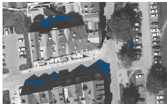
Figure 14. Part of the selected samples (blue squares) for the planarity control in shaded areas carried out for the Elblag test field (5 cm GSD) shown on the true orthophoto.
