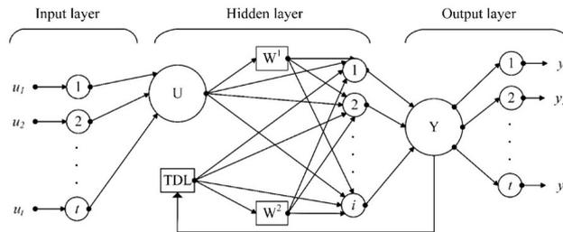
**Figure 2.** Architecture of a nonlinear auto-regressive neural network with exogenous input (NARXnn).
