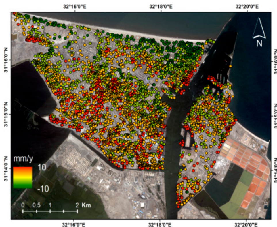
Figure 15. The average vertical ground motion velocities from 2007 to 2010 of pixels with coherence threshold \geq 0.3 .
