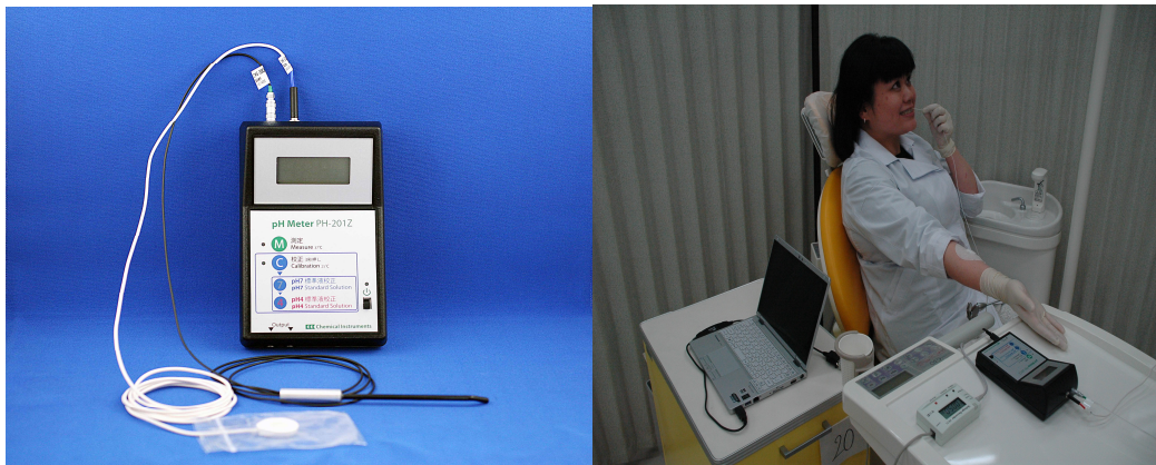
Figure 1. Measurement of enamel surface pH [13]. Left: pH antimony electrode connected to pH meter. Right: Photograph taken during enamel surface pH measurement.
