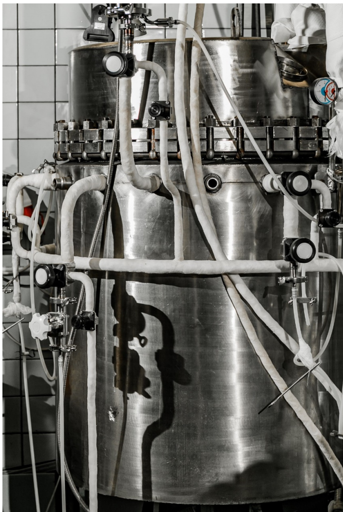
Supplementary Figure 1. Industrial scale bioreactors: 630-l (550 l working volume) bubble-type bioreactors of 1T series (CUC “EBEE”, Yoshkar-Ola, Russia) with air supply through ring-type gas distributor \varnothing 750 mm
