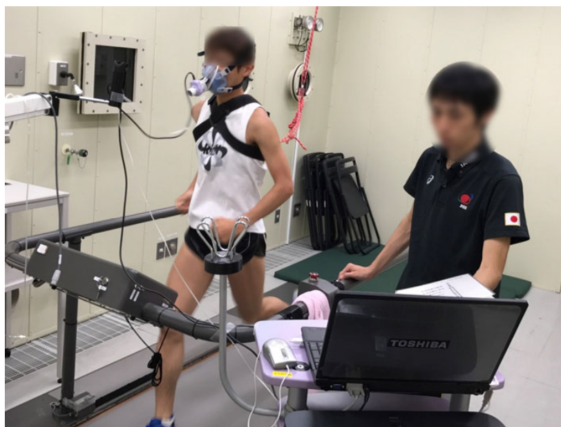
Figure 2. Indirect calorimetry using a face mask. Expired air was collected through a face mask, limiting the measurement duration to a few hours. The expired air was subjected to analysis of O 2 and CO 2 concentration.
