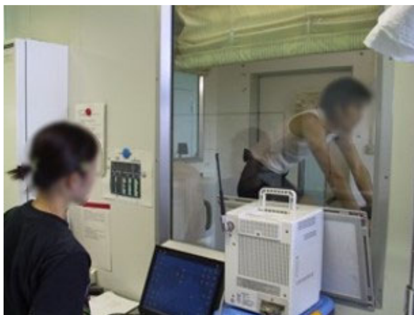
Figure 3. Whole-room indirect calorimetry. Changes in O_2 and CO_2 concentrations of the entire chamber are measured to assess O_2 uptake and CO_2 production of the participants without a mask and mouthpiece. This system, also known as a human calorimeter, allows us to track energy metabolism over time, including during sleep [37]. This method has limitations in assessing dynamic changes in energy metabolism caused by the dilution of the expired air with chamber air. Hence, efforts have been made to improve time resolution of the system [38].
