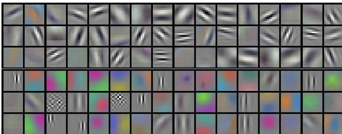
Figure 1. Example filters by Krizhevsky et al. [3]. Because these filters were learned using the first convolutional layer of the neural network, the represented features are simple, such as the edge orientation and frequency (learned features become progressively more complex with each additional convolutional layer). Reproduced with permission from Alex Krizhevsky, Advances in NIPS 25 ; published by Curran Associates, Inc., 2012.
