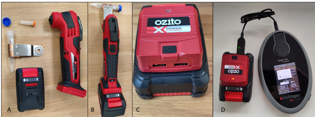
Figure 8. Field deployable sample preparation tools: (A) component parts of Osci-lyser, (B) the Osci-lyser assembled and ready to use, (C) USB adaptor for battery, providing 1.0- and 2.1-amp outputs, (D) Battery powering Qubit 2.0.
