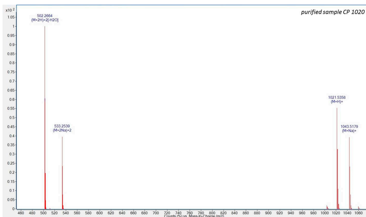
Figure 17. MS spectrum with charge carrier, neutral loss annotation and predicted isotope distribution (red bars) of CP1020.
