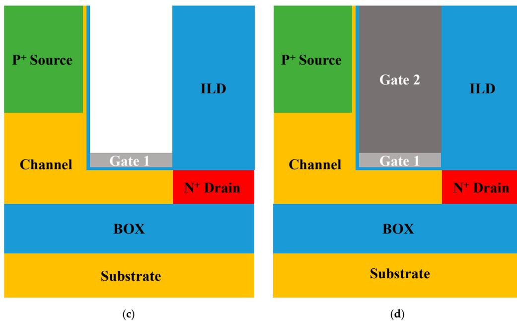
**Figure 9.** Key process steps for stacked gate L-shaped TFET. (a) Gate 2 is deposited by atomic layer deposition (ALD); (b) Gate 2 chemical mechanical polishing (CMP); (c) etch-back process; (d) Gate1 ALD & CMP.
