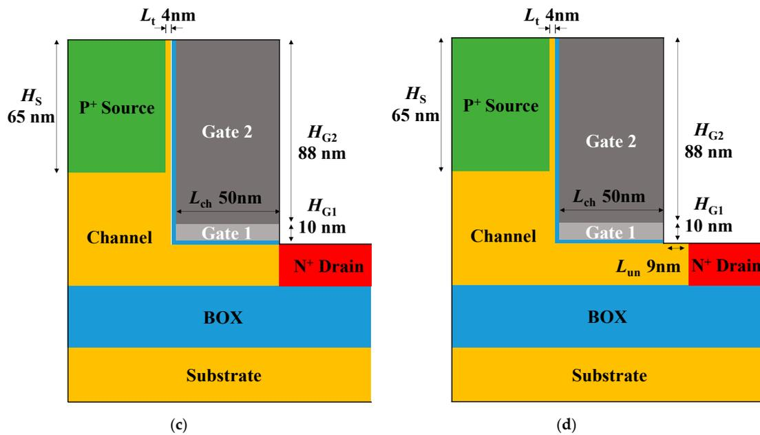
**Figure 1.** Schematic designs of (a) (conventional) single gate L-shaped tunnel field-effect transistor (TFET), (b) single gate L-shaped TFET with underlap, (c) stacked gate L-shaped TFET and (d) stacked gate L-shaped TFET with underlap. In order to compare the suppression of the ambipolar current for each method, the simulations were conducted according to the schematics above.
