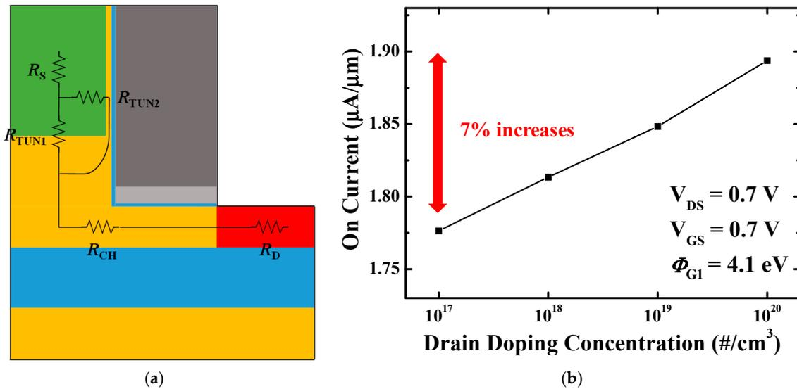
**Figure 8.** (a) Resistance network when the device is in the on-state.  $R_{TUN1}$  and  $R_{TUN2}$  are the tunneling resistances; (b) on-current with the drain doping concentration. After changed the source material to SiGe, 7% on-current increases with the drain doping concentration.
