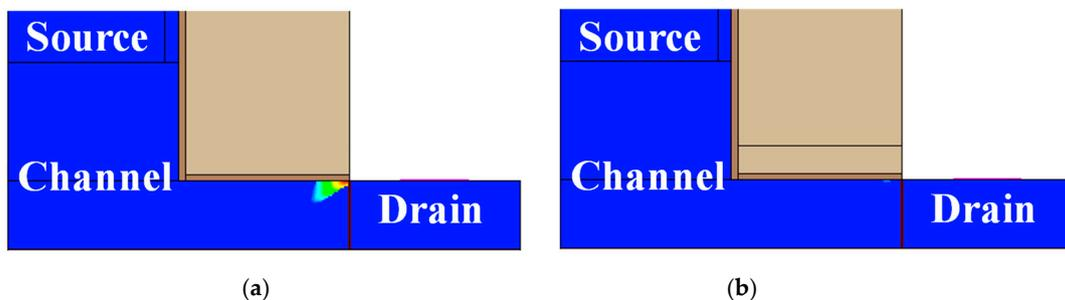
**Figure 3.** 2-D contour plot of band-to-band tunneling (BTBT) generation for (a) single gate and (b) stacked gate L-shaped TFET. Ambipolar current suppression is observed from the decreased BTBT rates in the stacked gate L-shaped TFET.
