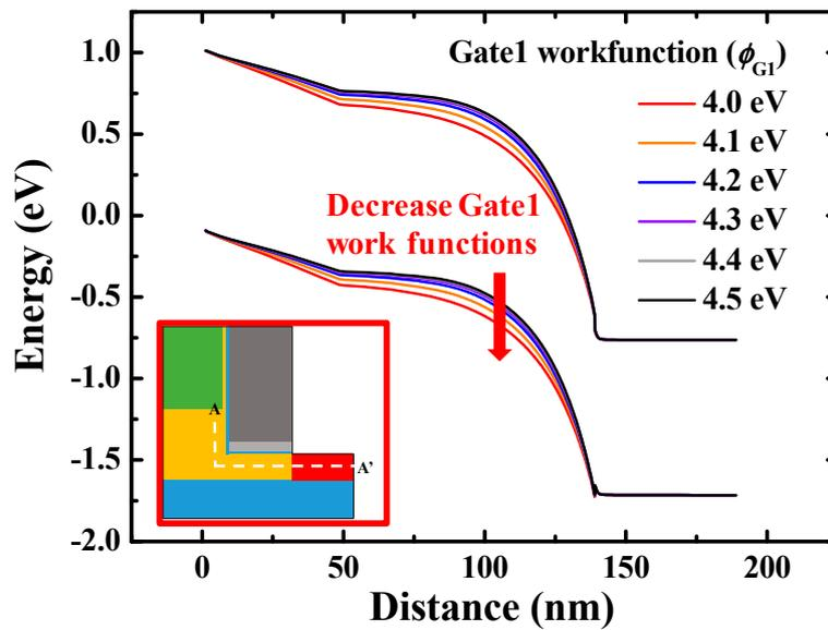
**Figure 6.** Energy band diagrams with various  $\phi_{G1}$  (at  $V_{DS} = 0.7$  V). They are obtained from channel-to-drain along the cutline which is indicated in the inset (A-A'). As  $\phi_{G1}$  decreases, the tunneling barrier between the channel and the drain becomes thicker.
