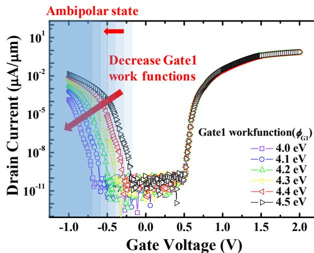
**Figure 5.** Transfer curves of stacked gate L-shaped TFET with various  $\phi_{G1}$  (at  $V_{DS} = 0.7$  V). As  $\phi_{G1}$  decreases, ambipolar current is suppressed more and also ambipolar state region contracts. It can be interpreted as if only the left part of the transfer curve ( $V_{GS} < 0$ ) is shifted to the left.
