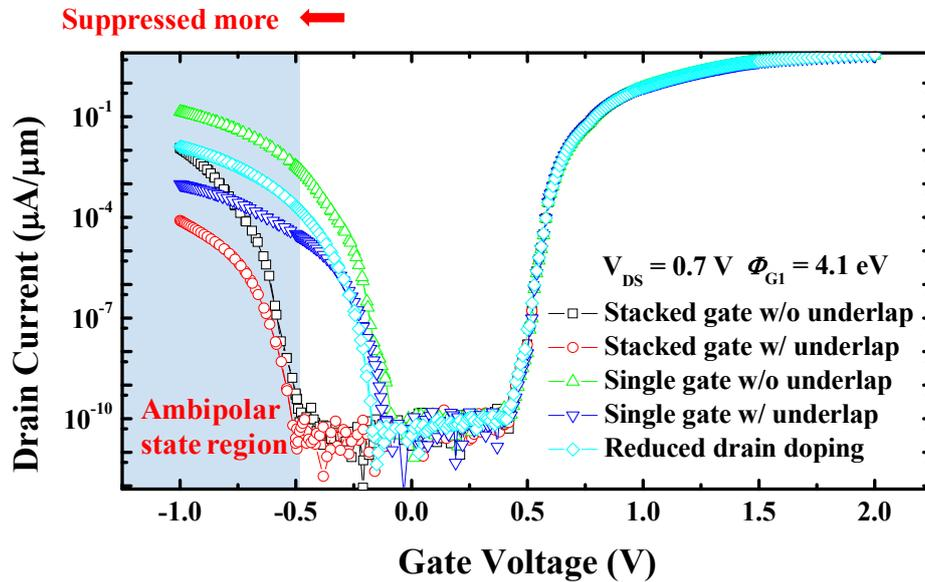
**Figure 4.** Transfer characteristics for stacked gate L-shaped TFET, stacked gate L-shaped TFET with underlap, low drain doping L-shaped TFET, (conventional) single gate L-shaped TFET, and single gate L-shaped TFET with underlap at  $V_{DS} = 0.7$  V. It is illustrated that the ambipolar state region significantly contracts in the stacked gate L-shaped TFET.
