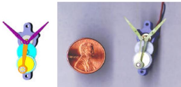
Figure 7. Internal transmission structure of Microbat.
