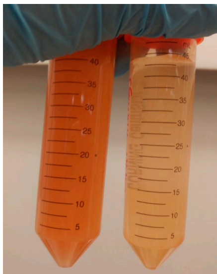
Figure S3B. Images of 50 mL sample (A) before and (B) after filtration using the \mu\text{FMS} device at 120 \mu\text{L/s} .
