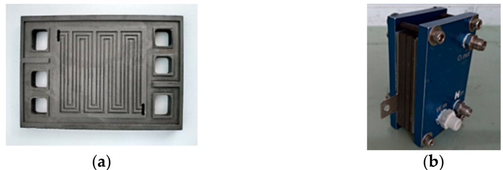
Figure 1. (a) Stereogram of runner plate; (b) fuel cell stack.
