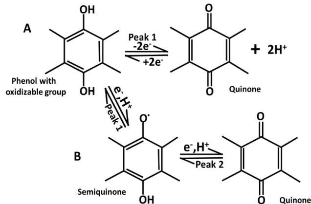
Figure S1. The chemical reaction process showing the oxidation of phenolic compounds having one peak in the reaction path (A) and the oxidation of phenolic compounds having two peaks in the reaction path (B).
