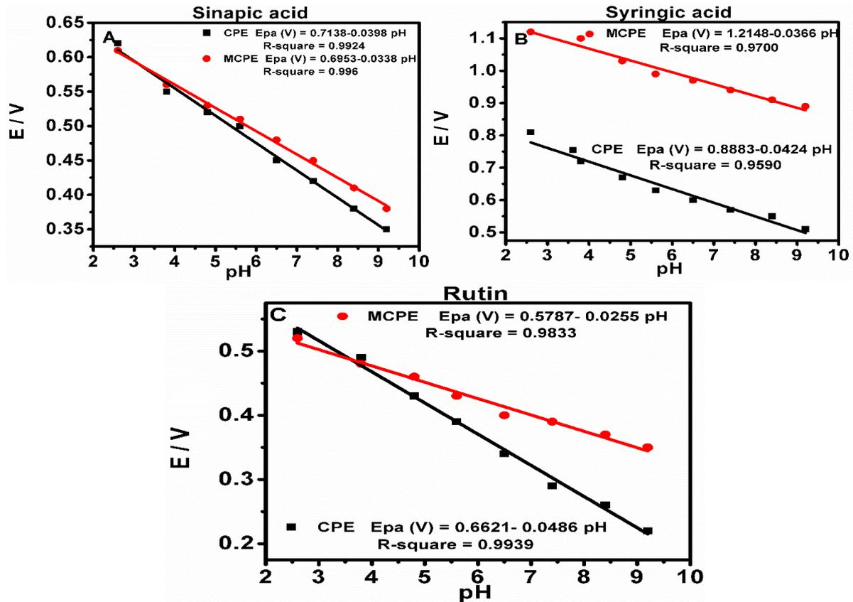
Figure S3. The linear regression plots for both CPE and MCPE to show the effect of pH on the electrochemical behavior of the phenolic compounds, in 0.5 M acetate buffer of pH 2.6, 3.8, 4.8, 5.6, 6.5, 7.4, 8.4 and 9.2, at a scan rate of 0.2 V/s.
