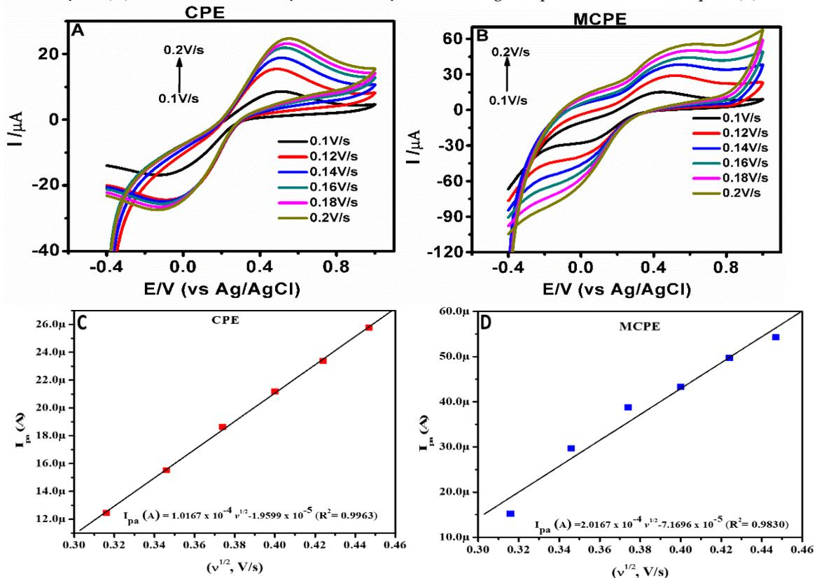
Figure S2. Cyclic voltammograms at (A) CPE and (B) MCPE, respectively in 1 mM K<sub>4</sub>[Fe(CN)<sub>6</sub>] of 0.1 M KCl by varying scan rates (0.1–0.2 V/s). The corresponding Plots of  $I_{pa}$  vs  $v^{1/2}$  at (C) CPE and (D) MCPE.
