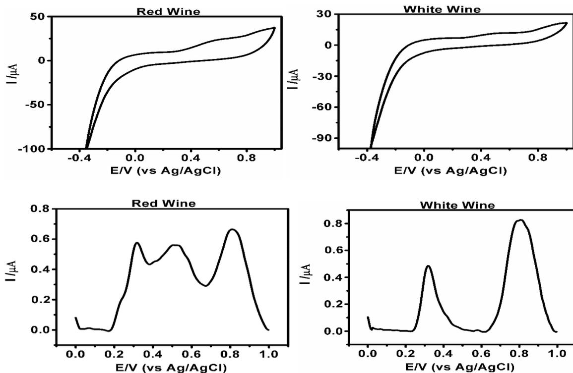
**Figure S9.** Cyclic voltammograms and Differential pulse voltammograms showing the determination of red and white wine real samples only using the modified electrode in 0.5M ABS pH 4.8 as supporting electrolyte.
