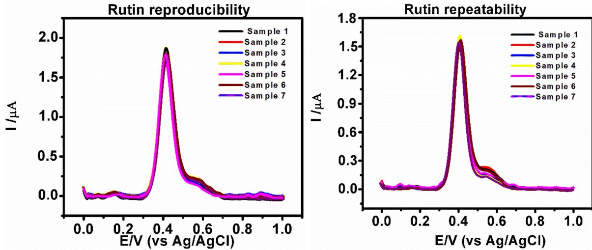
Figure S7. Differential voltammograms showing the reproducibility and repeatability of MCPE for the determination of the phenolic compounds respectively.
