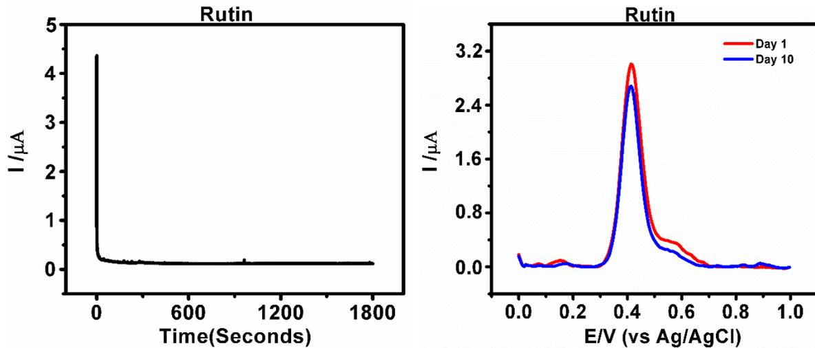
**Figure S8.** A steady amperometric current response for determination of stability of the sensor for phenolic compounds detection in (0.5 M ABS of pH 4.8), for 30 minutes, at MCPE using 0.6V potential. Differential pulse voltammograms shows the determination of  $0.9 \times 10^{-3}$  M for sinapic,  $1.0 \times 10^{-3}$  M for syringic and  $0.3 \times 10^{-3}$  M for rutin respectively in 0.5M ABS pH 4.8 for 1<sup>st</sup> day and 10<sup>th</sup> to show stability of the modified electrode.
