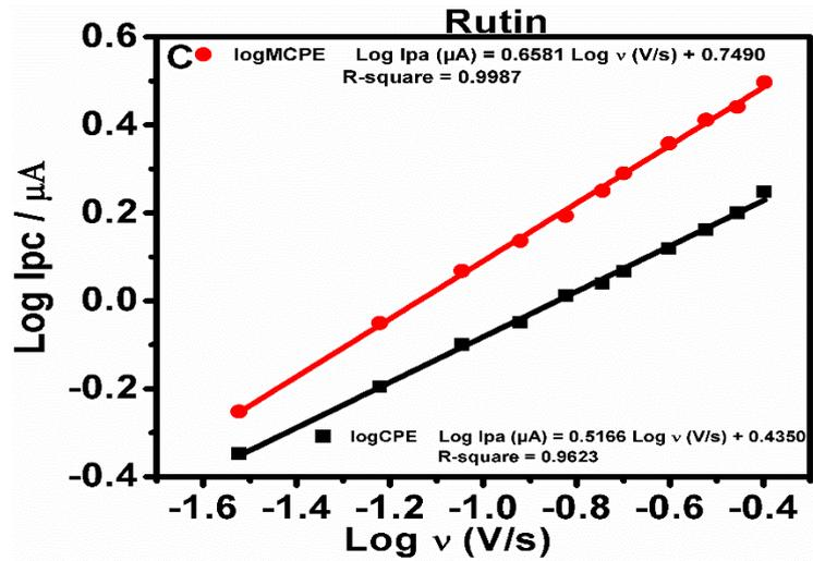
Figure S6. The linear relationship plots of logarithm of peak current and logarithm of scan rate ( $\log I_{pa}$  versus  $\log v$ ) for phenolic compounds. The plots, represents peak current and logarithm of scan rate at CPE and MCPE.
