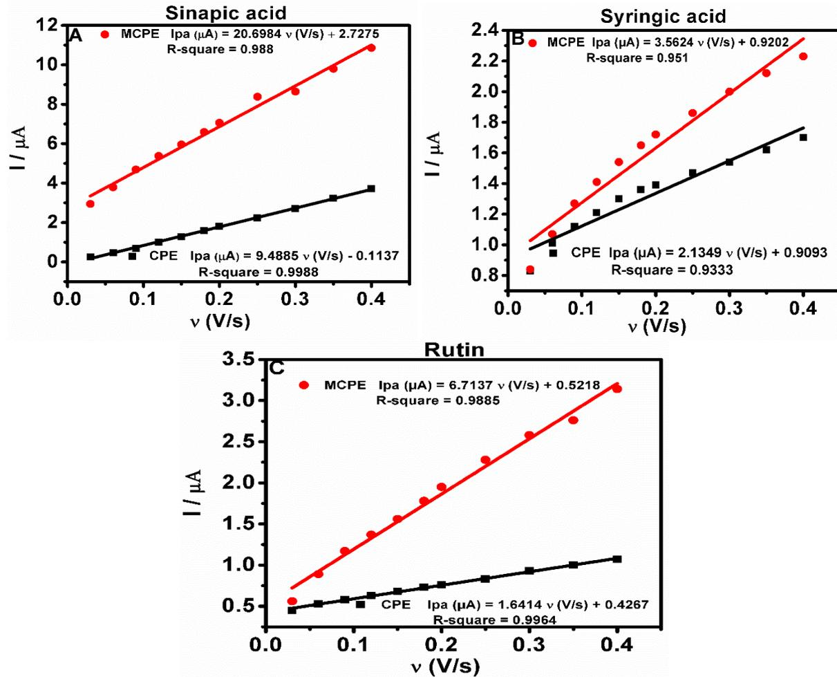
**Figure S5.** Linear regression plots showing the dependence of redox (anodic and cathodic) peak current on scan rate  $I_p$  versus scan rate  $v$  (V/s) for controlled adsorption. The plots, represents controlled adsorption at CPE and MCPE in 0.5 M of ABS with pH 4.8, scan rate of 0.03, 0.06, 0.09, 0.12, 0.15, 0.18, 0.20, 0.25, 0.3, 0.35 and 0.40 V/s respectively with a reversible scanning potential range of -0.4 to 1.0 V.
