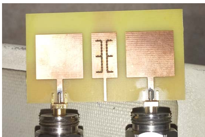
Figure 10. Photograph of the fabricated antenna array with slotted MTM-DS.
