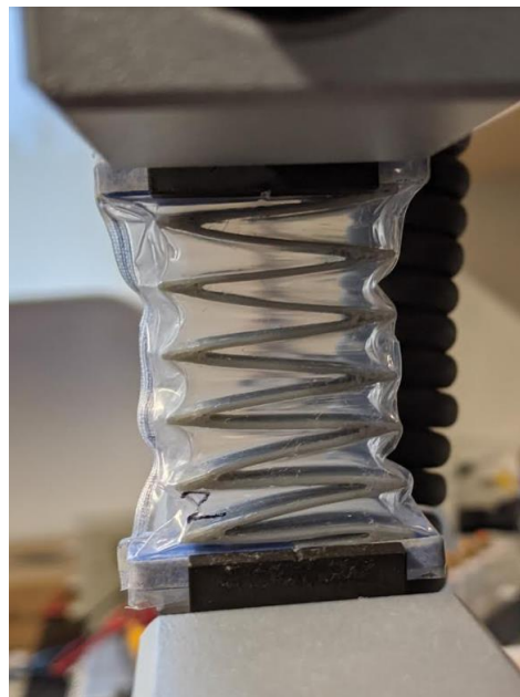
Figure S2. Image of partially-contracted actuator under vacuum, particularly to illustrate the small sections of actuator skin in between the skeleton gaps. These provide increased reaction forces particularly at the end of the contraction, and so are relevant to the reaction force measurement.
