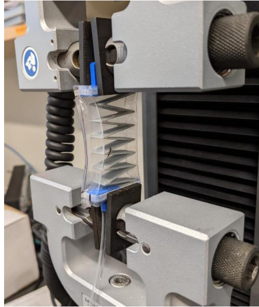
Figure S1. Experimental setup for force-contraction profile measurement experiment on mechanical tester.
