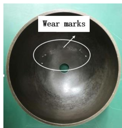
Figure 13. Schematic diagram of rotor wear.
