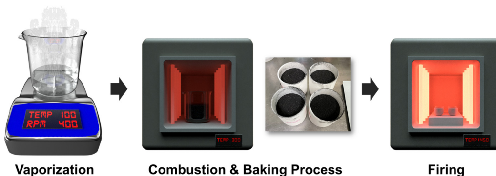
Figure 1. Schematic of the manufacturing process of nano phosphors through sol-gel combustion.
