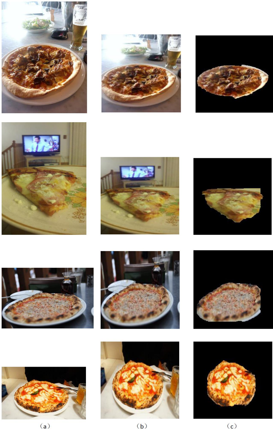
Figure 11. GrabCut-based segmentation experiment results for pizza objects in COCO dataset: (a) original input image; (b) image after resizing; (c) GrabCut method segmentation results.
