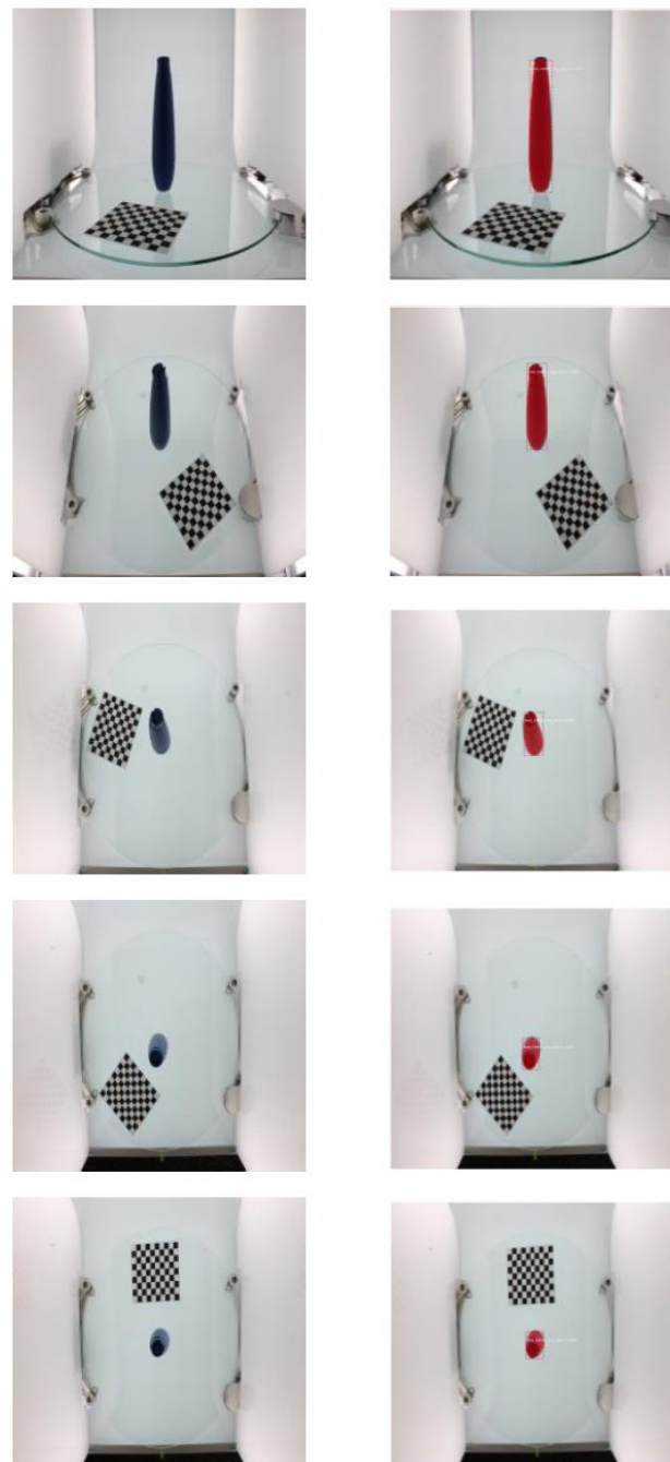
Figure 12. Results for ikea_table_leg_blue data using the Mask R-CNN-based object detection method. The column on the left contains the input images. The column on the right shows the positioning and segmentation results.
