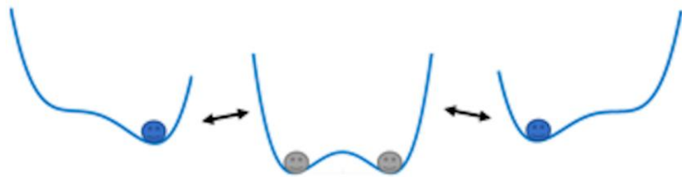
Figure 4. Diagram of stochastic resonance effect of bistable system.
