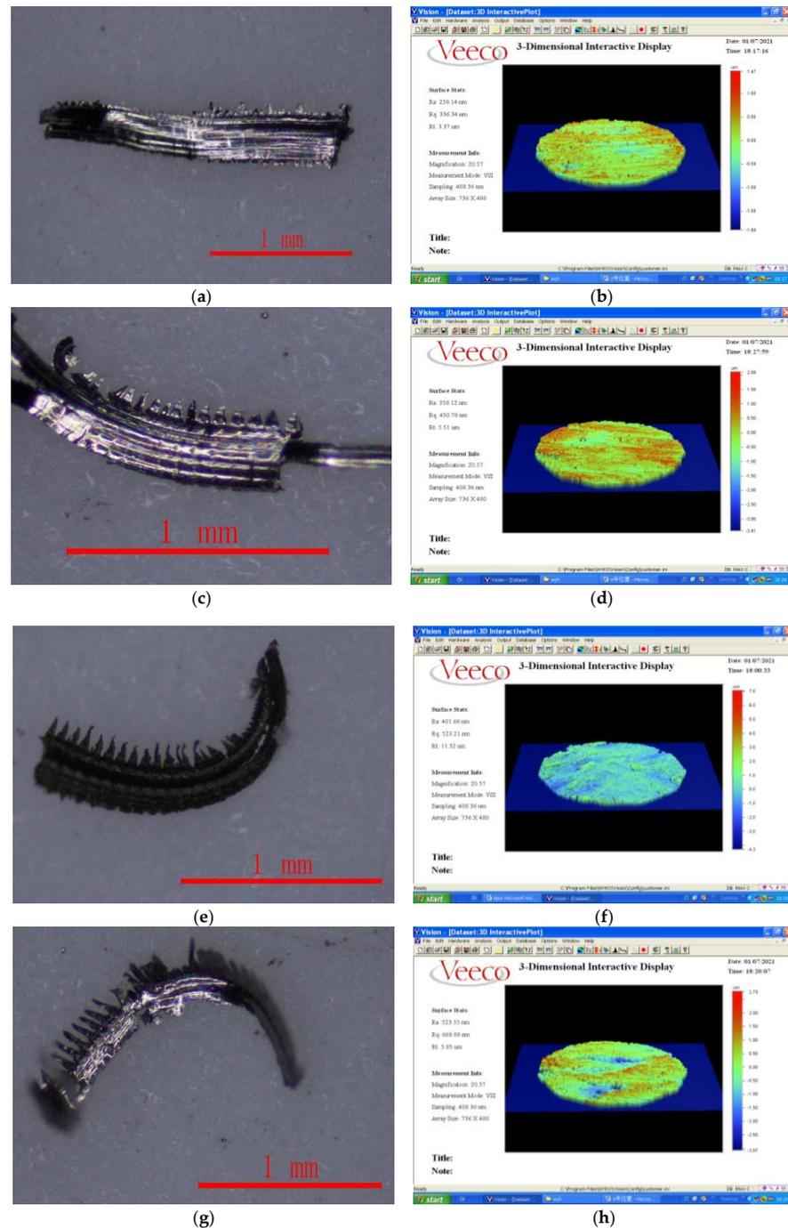
**Figure 10.** The shape of chips and roughness of surface. (a) Chip topography (Cutting force is 280 N). (b) Three-dimensional surface topography. (c) Chip topography (Cutting force is 400 N). (d) Three-dimensional surface topography. (e) Chip topography (Cutting force is 470 N). (f) Three-dimensional surface topography. (g) Chip topography (Cutting force is 620 N). (h) Three-dimensional surface topography.
