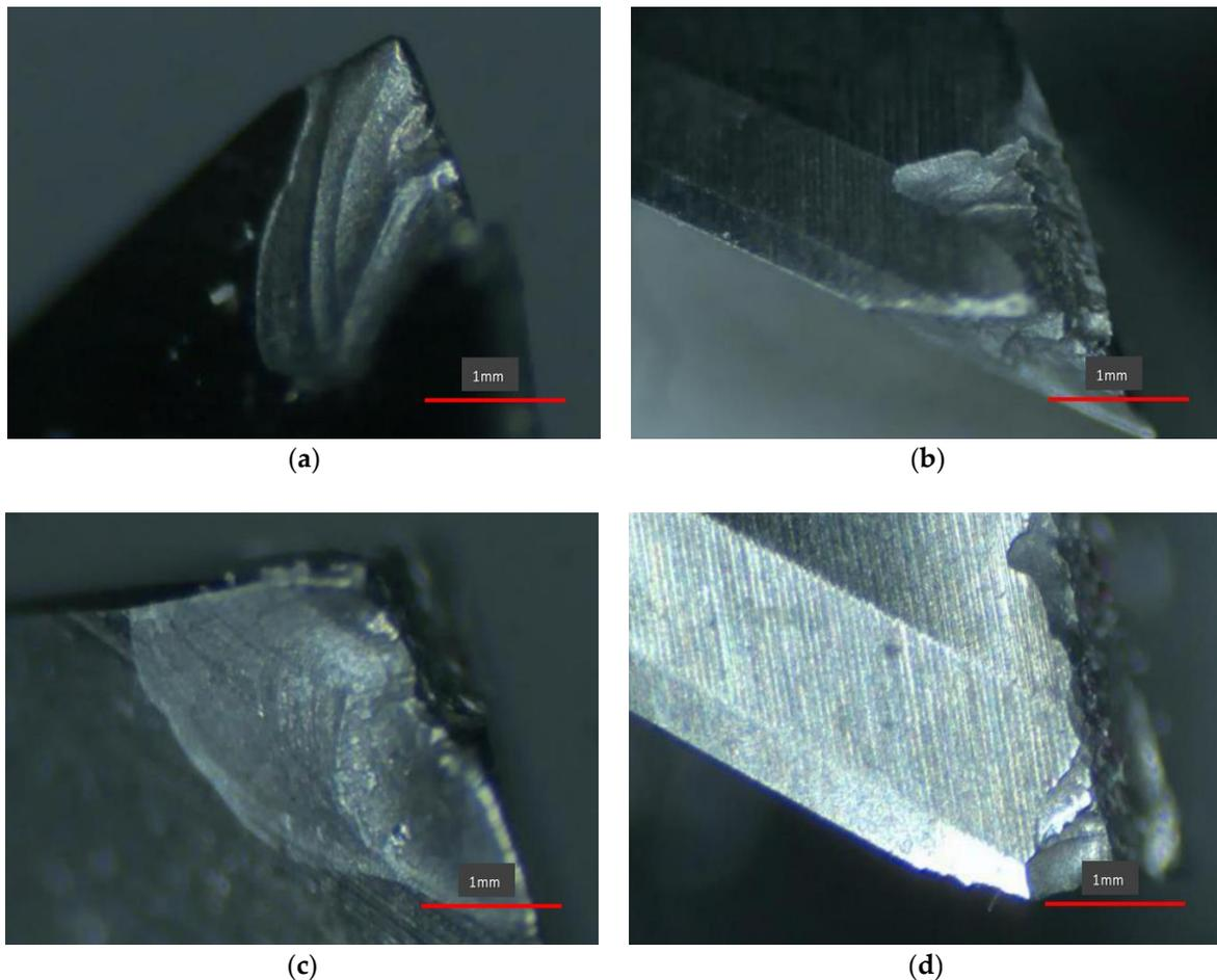
**Figure 11.** Wear morphology of tool. ( $n = 300$  r/min,  $a_p = 0.4$  mm,  $f_z = 0.4$  mm/r). (a) Wear morphology of flank face. (b) Wear morphology of rake face. (c) Layered flaking. (d) Tool chipping.
