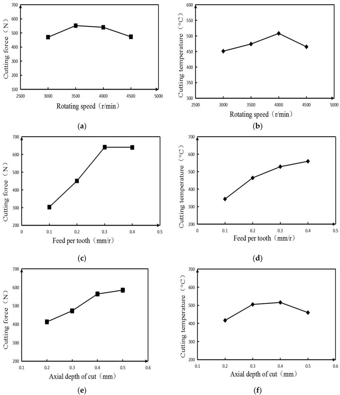
**Figure 2.** Trend chart of indicator factors. (a) The influence of spindle speed. (b) The influence of spindle speed on cutting force on cutting temperature. (c) The influence of feed per tooth. (d) The influence of feed per tooth on cutting force on cutting temperature. (e) Influence of axial depth of cut. (f) Influence of axial depth of cut on cutting force on cutting temperature.
