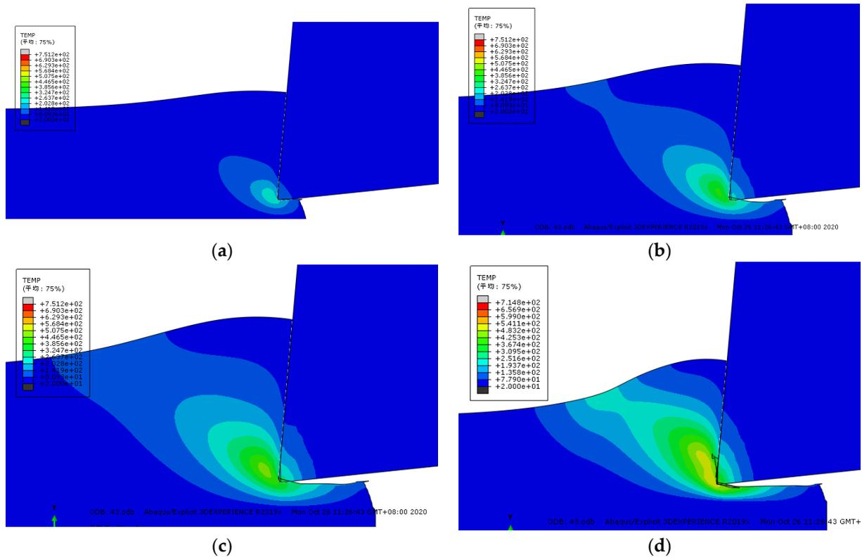
**Figure 8.** Changes in the cutting temperature field at the beginning of cutting ( $^{\circ}\text{C}$ ). (a)  $t = 5 \times 10^{-4}$  s (b)  $t = 8.8 \times 10^{-4}$  s. (c)  $t = 1.2 \times 10^{-3}$  s (d)  $t = 2.2 \times 10^{-3}$  s.
