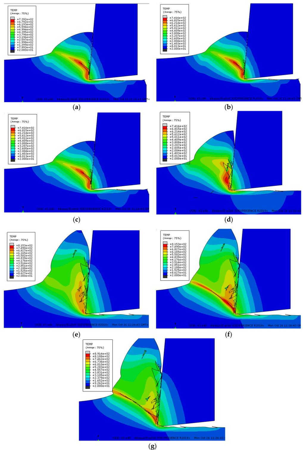
**Figure 9.** Changes in the cutting temperature field during the formation of serrated chips ( $^{\circ}\text{C}$ ). (a) The first section is about to be formed. (b) The first block is fully formed. (c) The second block begins to form. (d) The second nodal development process. (e) The second nodal mass starts to slip. (f) The second nodal slip process. (g) The second block is fully formed.
