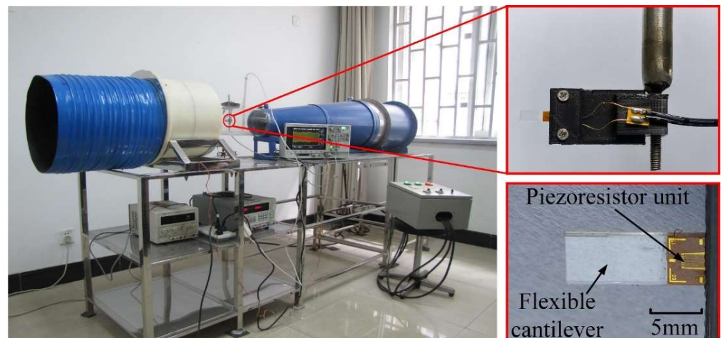
Figure 3. Schematic diagram of the measurement setup and the photograph of the fabricated microcantilever anemometer prototype.
