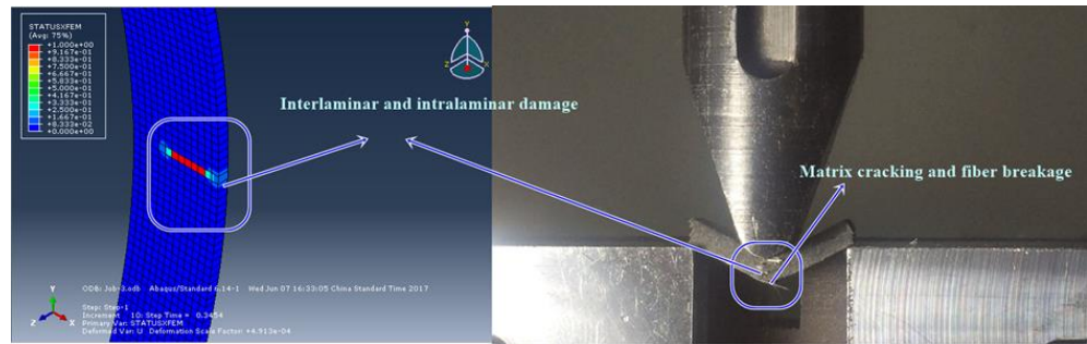
Figure 10. XFEM damage comparison for 3P/0° specimen.
