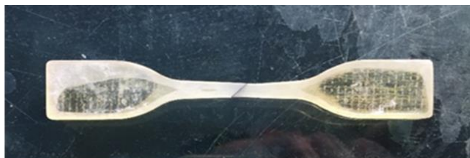
Figure 7. Grinding qualified resin matrix spline.
