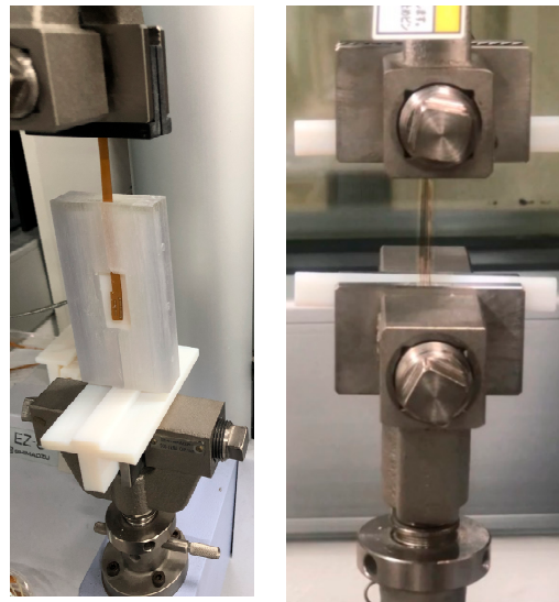
Figure 3. Tensile tests of the FPCB and PSPI test samples.
