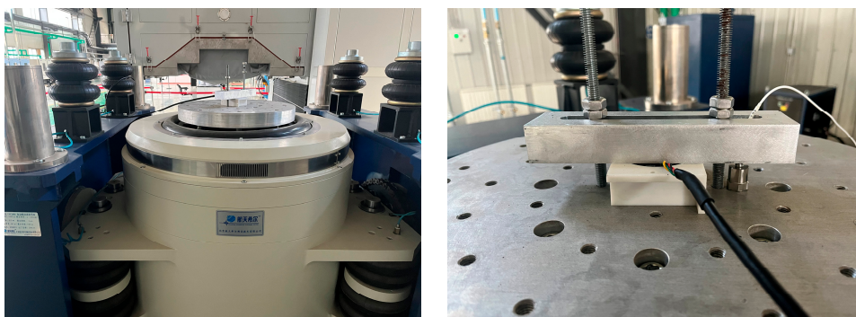
Figure 5. Acceleration sensor dynamic calibration test.
