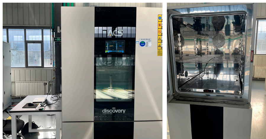
Figure 7. Temperature drift experiment for the acceleration sensor.
