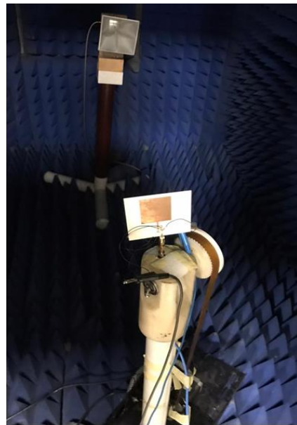
Figure 13. The setup of the radiation patterns measurements of the filtenna.
