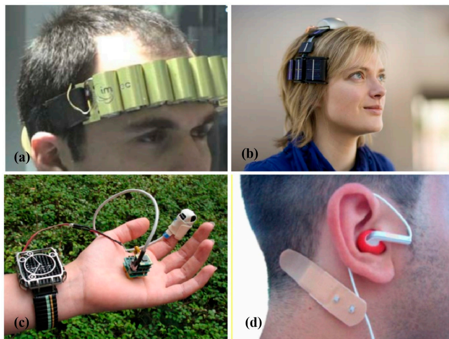
Figure 6. (a) Thermal power supply wireless EEG on the headband. (b) Wearable headset-type wireless EEG system with hybrid power supply. Reprinted with permission from [38]. Copyright 2009, IEEE-INST ELECTRICAL ELECTRONICS ENGINEERS INC. (c) “Watch” type TEG (left), an electronic device with a wireless module (center), and a commercial finger pulse oximeter (right). (d) Biomedical hearing aids.
