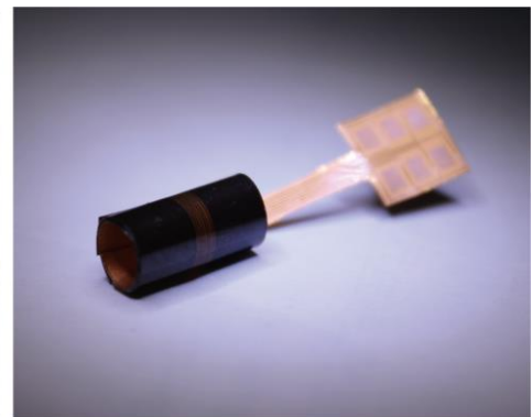
(d) The substrate was further rolled in the longitudinal direction. A circular tube with double outer circle was formed.
