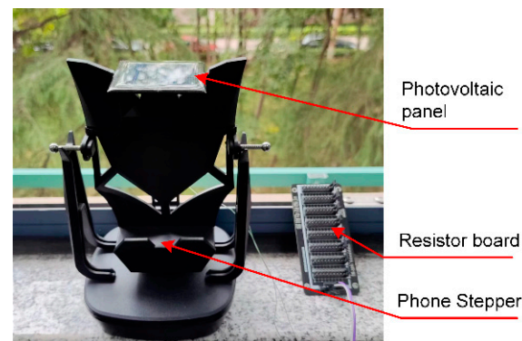
Figure 5. Experimental measurements of micro-power photovoltaic panels under dynamic condition.
