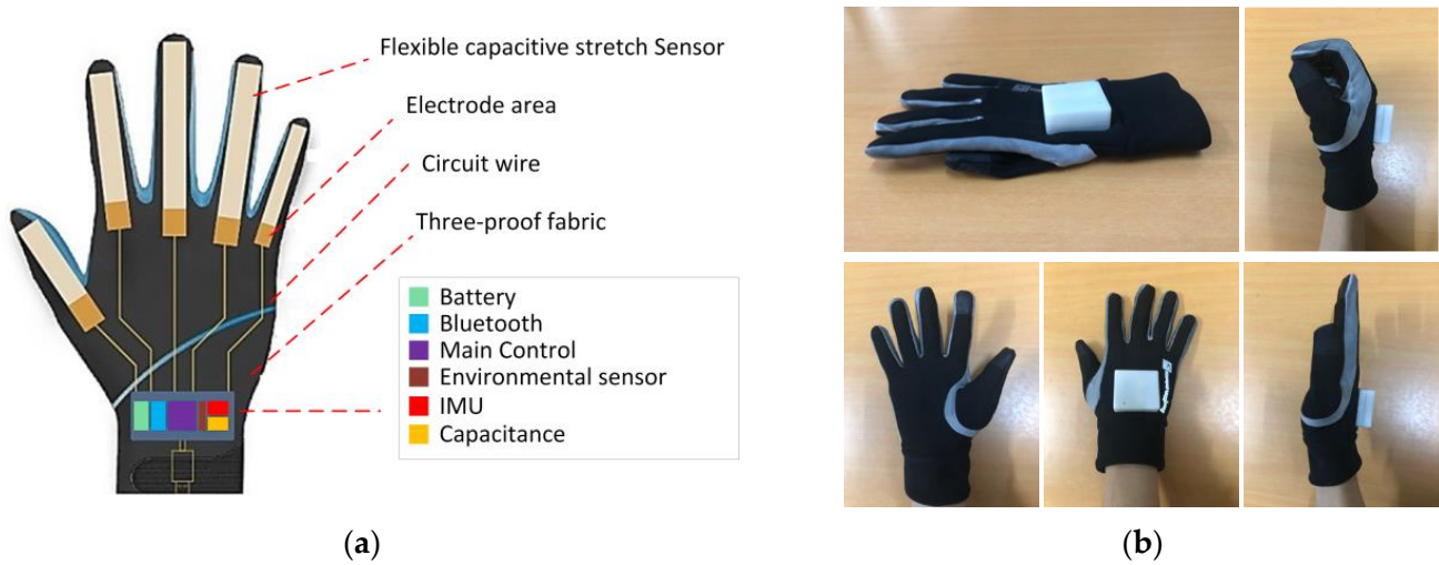
Figure 1. Proposed smart data glove: (a) structure diagram, (b) appearance.
