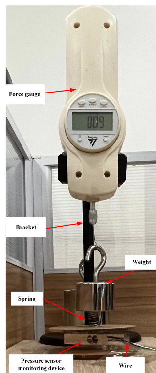
Figure 7. Experimental device diagram for analyzing the monitoring accuracy of flexion force value.
