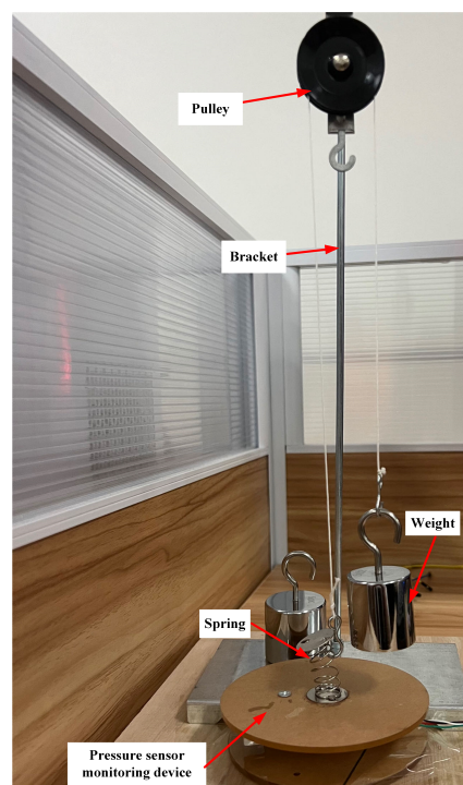
Figure 6. Experimental device diagram for analyzing the monitoring accuracy of extension force value.
