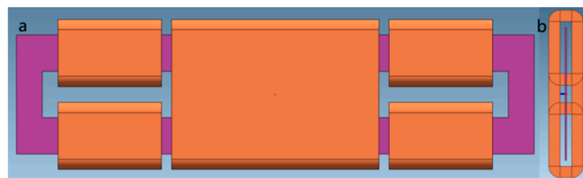
Figure 4. Simulation model of the fluxgate. (a) top view of the model. (b) side view of the model.
