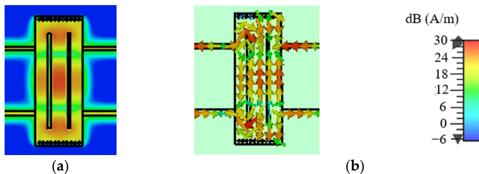
Figure 3. The surface current distributions on the SIW with two slots for DM operating at f_0 . (a) The uniform amplitude distributions. (b) The vector distributions.
