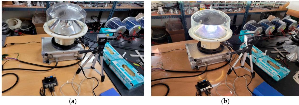
Figure 14. (a,b) Change in light intensity according to sea fog concentration value input.
