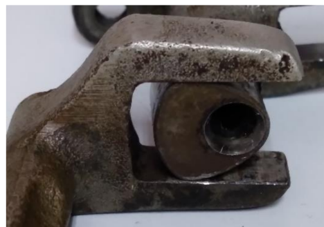
Figure 2. Photograph of the constant-breath cam mechanism with a flat-faced double-oscillating follower, used in a traditional sewing machine.
