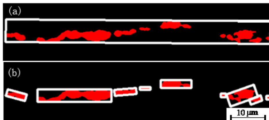
Figure 7. Establishing the length (a) and width (b) by forming the minimum bounding rectangle.
