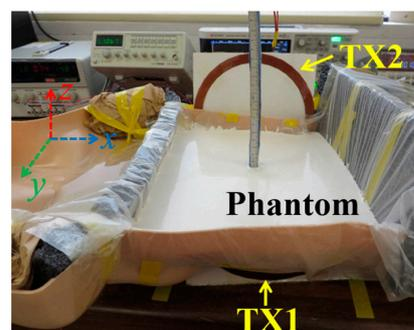
**Figure 5.** Liquid phantom for capsule localization investigation [70]. Reproduced with permission from an open-access article from *IEEE Access* (CC-BY).
