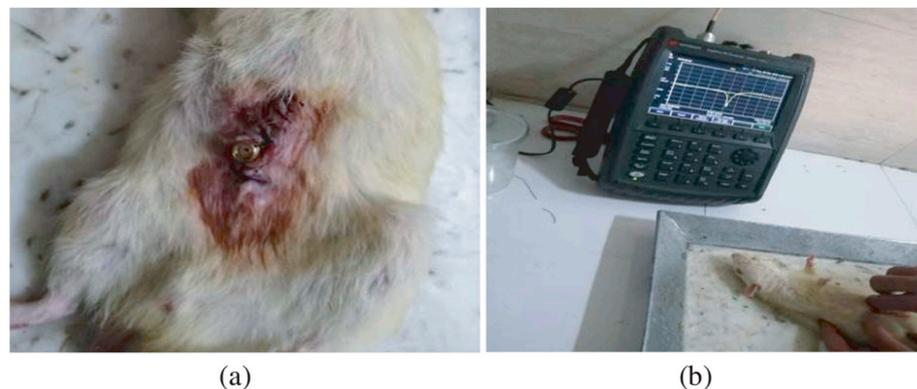
**Figure 7.** Multi-layer implantable antenna measurement for continuous glucose monitoring. (a) A sensor implanted in a rat, (b) Experimental setup [77]. Reproduced by courtesy of the Electromagnetics Academy.
