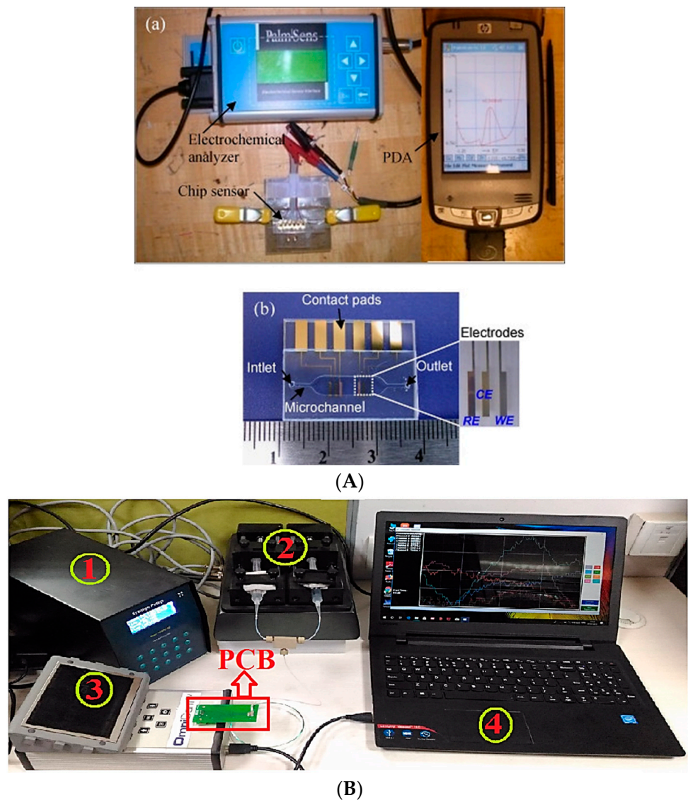
Figure 11. (A) Images (a) of the experimental set up for on-site measurement of Cd 2+ and (b) of the disposable polymer lab chip with the microchannel and the integrated electrochemical sensor. Reproduced with permission from reference [118]. (B) Image of the portable experimental set up for Cd 2+ detection in ground water using a microfluidic platform consisting of a microcantilever-based piezoresistive sensor. (1 and 2) are used for the flow control (syringe pump and controller), (3) the piezoresistive module and (4) the interface software running on a PC. Reproduced with permission from reference [123]. This article is published under a CC BY license.
