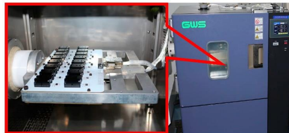
Figure 9. Accelerometer temperature performance test system.
