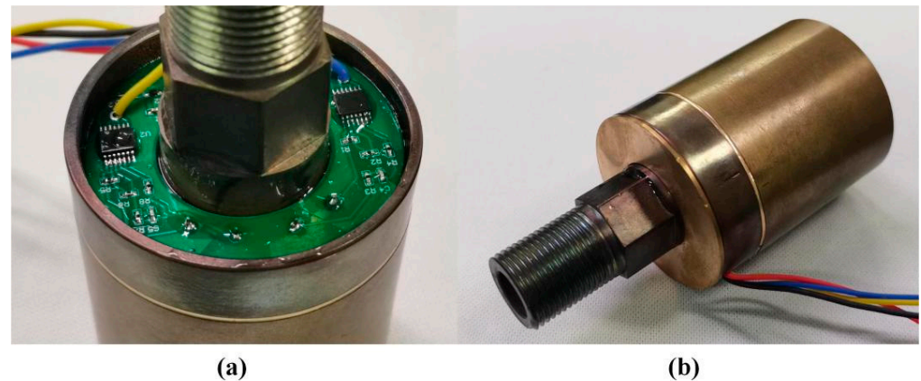
Figure 13. Physical image of sensor prototype: (a) Circuit lower chamber; (b) Cap packaging.
