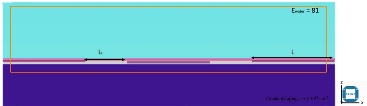
**Figure 5.** Schematic of the FET from the X, Z view for electrical characterisation, with channel length ( $L_c$ ) and electrode length ( $L$ ).
