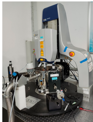
Figure 10. Polytec MSA-600-VD scanning laser vibration measurement and modal analysis system.
