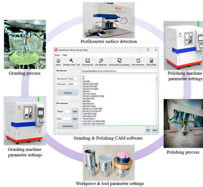
Figure 12. Closed-loop error compensation with CAM software.
