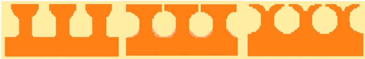
**Figure 13.** Typical cross sections of reentrant cavities used in pool boiling. Adapted from [111].
